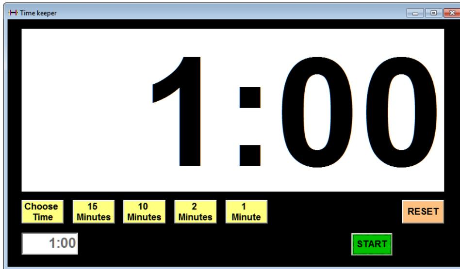
The operation of TMK is fairly self-evident. There are buttons to set specific times and any time up to 59:59 may be set by use of the “Choose Time” button. When active (counting down) the only button visible is “Stop”.
